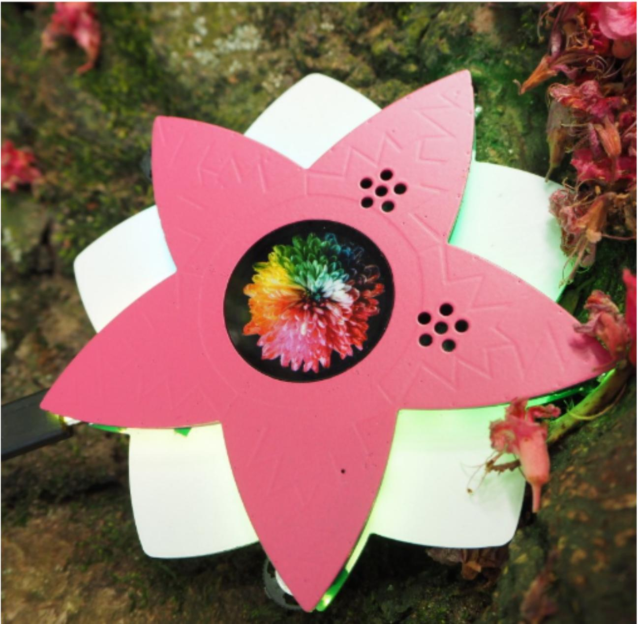
Figure 7: CCC 2023—Flow3r strumento musicale programmabile in microPython
